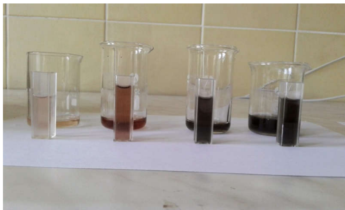
Figure 1. Change in colour indicates the presence of silver nanoparticles, hereby using the apple extract. (Personal source)
