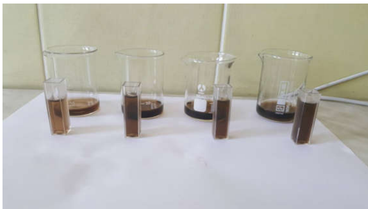
Figure 2. Synthesized nanoparticles using the extract of banana. (Personal source).
